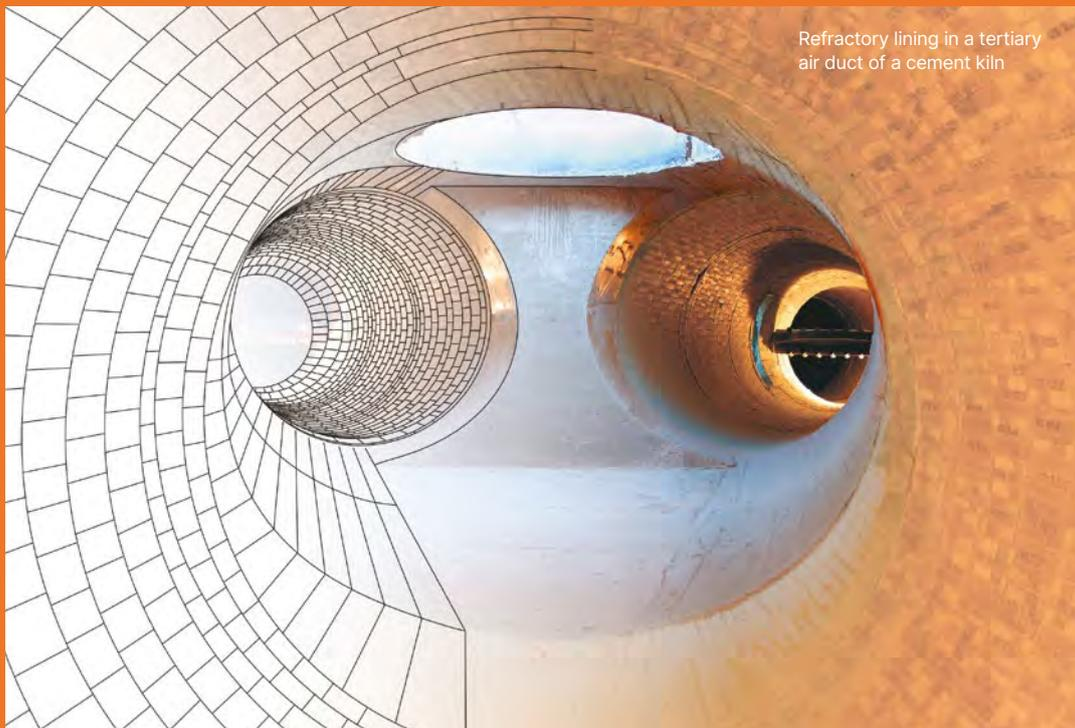
Refractory lining in a tertiary air duct of a cement kiln
