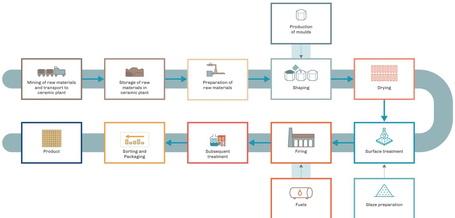
\* Simplified diagram of the stages in the manufacture of ceramic products. The production process may vary according to the correspondent Ceramic sub-sector.
